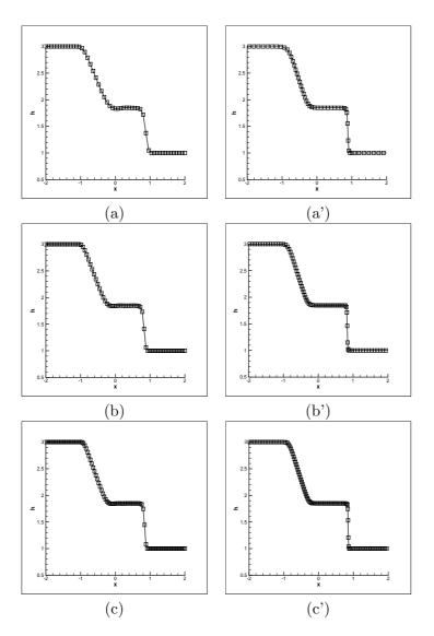
FIGURE 3. Height: (a),(b), and (c) show numerical solutions by MUSCL of J = 50, 75, and 100, respectively. (a'),(b'), and (c') show numerical solutions by MUSCL with MMM of J = 50, 75, and 100, respectively.
