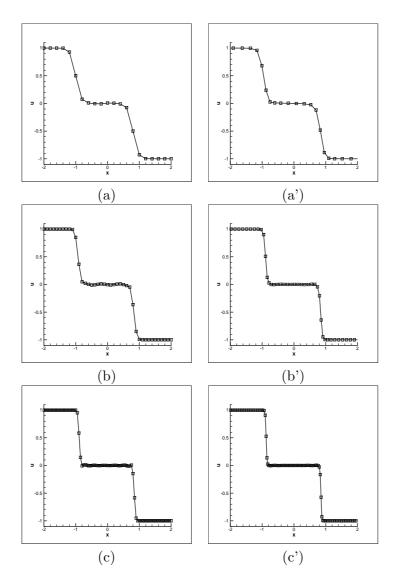
FIGURE 7. Velocity: (a),(b), and (c) show numerical solutions by MUSCL of J = 20, 40, and 80, respectively. (a'),(b'), and (c') show numerical solutions by MUSCL with MMM of J = 20, 40, and 80, respectively.
