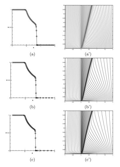
FIGURE 2. (a),(b), and (c) show numerical solutions by MUSCL with MMM of monitor parameter 1, 10, and 20, respectively. (a'),(b'), and (c') show mesh trajectories of monitor parameter 1, 10, and 20, respectively. (J=50)
