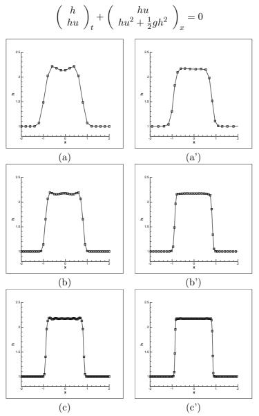
FIGURE 6. Height: (a),(b), and (c) show numerical solutions by MUSCL of J = 20, 40, and 80, respectively. (a'),(b'), and (c') show numerical solutions by MUSCL with MMM of J = 20, 40, and 80, respectively.
