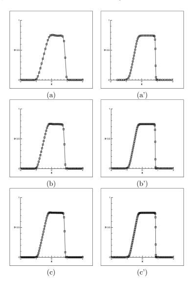
FIGURE 4. Velocity: (a),(b), and (c) show numerical solutions by MUSCL of J = 50, 75, and 100, respectively. (a'),(b'), and (c') show numerical solutions by MUSCL with MMM of J = 50, 75, and 100, respectively.
